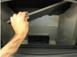
3. Lift up on one of the side panels to release the (2) tabs on the bottom of the panel from the notches in the firebox. Guide the bottom of the panel forward until it can be lowered into the ashpan area.
