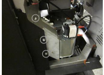
Disconnect the blower assembly (the wiring may remain in place during cleaning. Clean all dust and debris from the convection blower.
