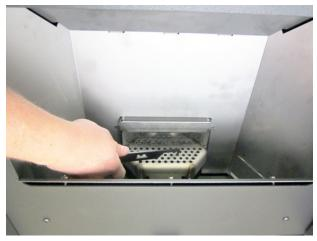
4. Brush away flyash around the burn platform using the brush included with the stove. The flyash will fall into the ashpan below.
