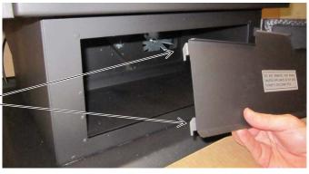
2. Remove the exhaust channel cover plate and gasket (a single wingnut holds it in place). When replaced, make sure the gasket on the cover plate seals the cover plate against the exhaust channel.
