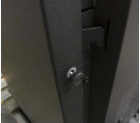
3. Slide the side panel back, tilt it outwards, and remove it from the stove. Note how the panel is held in place with three tabs on the back.
