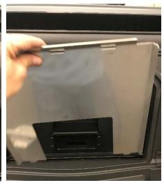
7. With the liners removed, clean all flyash and debris from the firebox. Clean the liners before replacing. Make sure to clean the heat exchanger on the firebox ceiling.
