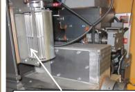
Impellers are accessible for maintenance without removing blower.
