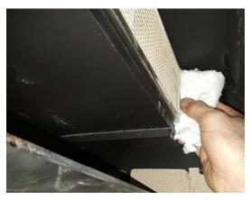
2. Grab both edges of the combustor and work it out by pulling back and forth on both sides.
