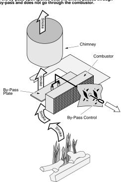
With the by-pass closed (pushed in), the smoke passes through the combustor.
