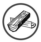
This fireplace was designed to burn solid wood fuel only (cord wood). Never use treated wood, wax logs, coal, garbage, or other materials. These materials will void the safety listing and may damage the combustor.
