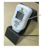
Press this ON/HOLD button to view the temperature
