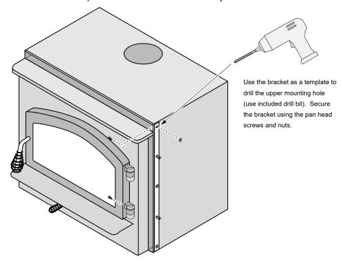
4. Place the insert into position (flue attached). Attach the surround panel as shown below.
