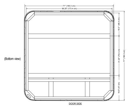
**NOTE: WATKINS WELLNESS** recommends that the SX be installed on a minimum 4" (10.2cm) thick reinforced concrete pad or structurally sound deck able to support the "dead weight" found in the spa specification chart. **IMPORTANT:** THE SX MUST NOT BE SHIMMED IN ANY MANNER.
