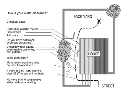
If the spa has to be taken off of the cart to go over a wall (either because the entry area is too narrow, the eaves are too low, the corner is too tight, or the stairway is too steep), a crane will be required. Don't be alarmed!
