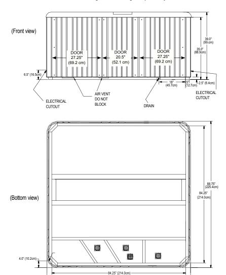
**NOTE: WATKINS WELLNESS** recommends that the Tempo be installed on a minimum 4" (10.2cm) thick reinforced concrete pad or structurally sound deck able to support the "dead weight" found in the spa specification chart.
