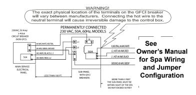
wiring access panel of the control box. A licensed electrician should install a four-wire electrical service (two line voltages, one neutral, one ground) from the main electrical service panel to the subpanel.
