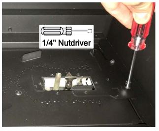
Remove the burner and place it aside.
