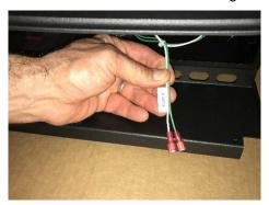
Connect the Green and White wires from the back of the remote to the "REMOTE" wires found in step
