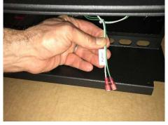
Connect the Green and White wires from the back of the remote to the "REMOTE" wires found in step
