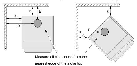
**Clearance Requirements: Mobile Home Clearance** 13" Α Sidewall to stove 330mm В 4-1/4" Backwall to stove 108mm C Cornerwall to stove 6-1/2" 165mm D Connector to sidewall 21-1/2" 546mm Ε 6-1/2" Connector to backwall 165mm F 15" Connector to cornerwall 381mm
