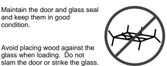
Do not use a grate or other device to elevate the fire off of the firebox floor. Burn the fire directly on the bricks.
