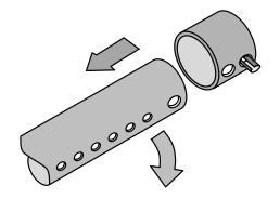
Slide the air tube to the left, swing it down and remove from the firebox.
