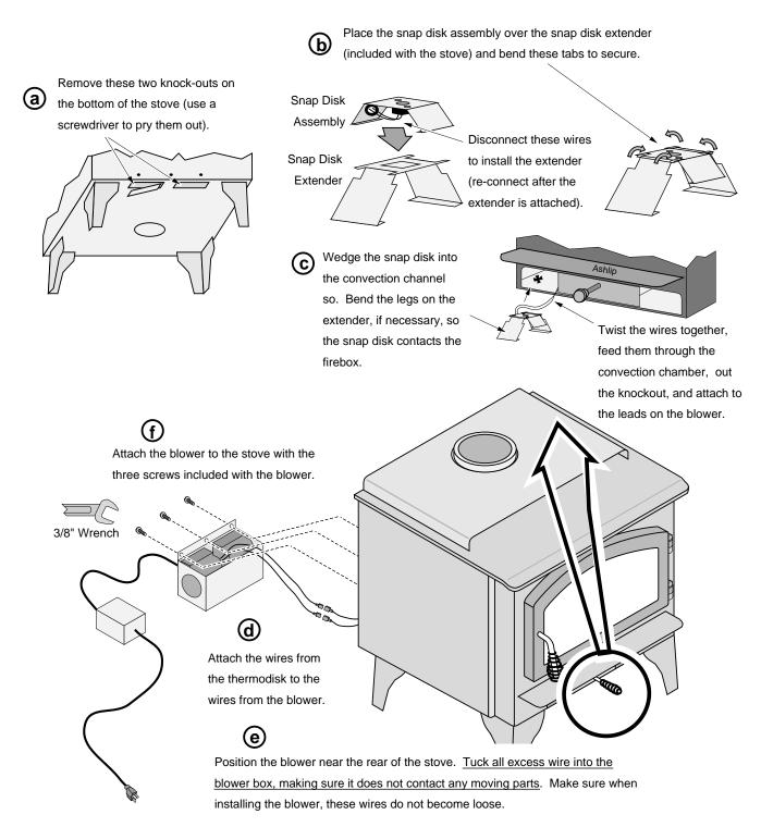
Plug the blower in. Do not route the power cord under or over the stove or in a location where it may become damaged.
