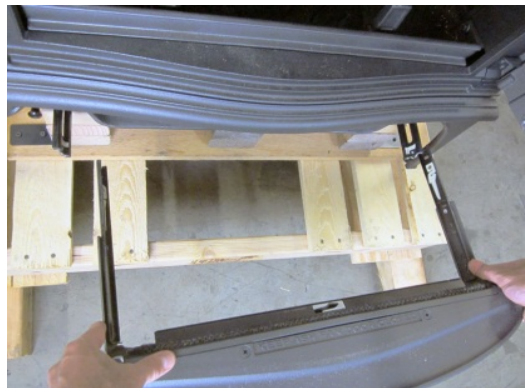
Ash Pan Drawer - Push the inside lift clip down, right clip up, then slide out.
