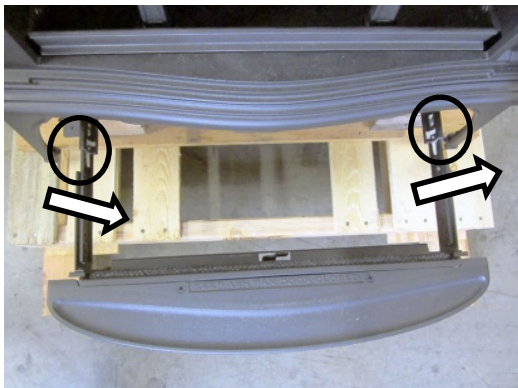
Ash Pan Drawer - Push the inside lift clip down, right clip up, then slide out.
