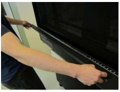
2. Remove the three screws holding the screen in place (1/4" nutdriver- magnetic driver recommended). Then pivot the screen down slightly until the clips on the bottom disengage from the glass frame.
