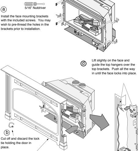
Make sure the door does (C) not open while installing.
