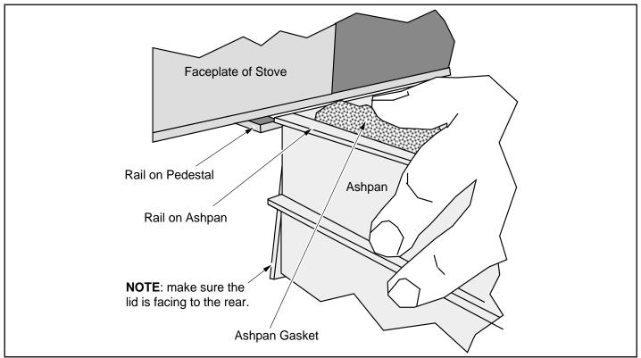
**3** Rotate the handles on both sides of the pedestal forward. The handles, when rotated, compress the ashpan against the stove and create an air-tight seal between the ashpan and stove. If you do not feel the handles compress, check alignment of the ashpan.
