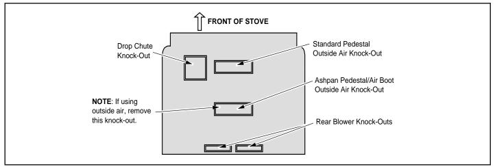
**3** Open the door to the stove and remove the floor firebricks on the left side. Locate the drop chute cover on the floor of the firebox. Remove the four bolts that secure it with a 7/16" wrench. Remove the cover and the gasket below it. Insert the drop chute gasket around the drop chute. Then insert the drop chute through the hole in the firebox floor. Position the drop chute so the slots run side to side. Replace the four bolts to secure the drop chute.
