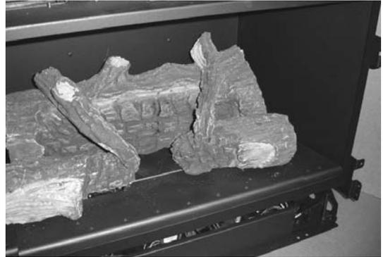
The right twig has a single hole on the bottom that fits over the pin on the rear log. Place the twig as shown above, noting how the twig points towards the center.
