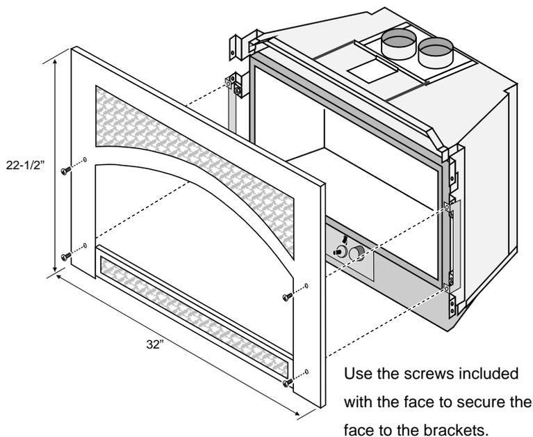
**WARNING:** When attaching the Victorian Lace Face, **do not over-tighten the screws.** Over-tightening the screws may damage the face – simply tighten the screws until they contact the face.
