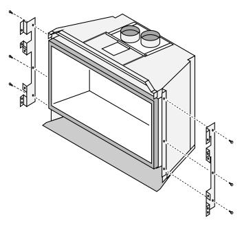
Attach the mounting brackets included with the backing plate.
